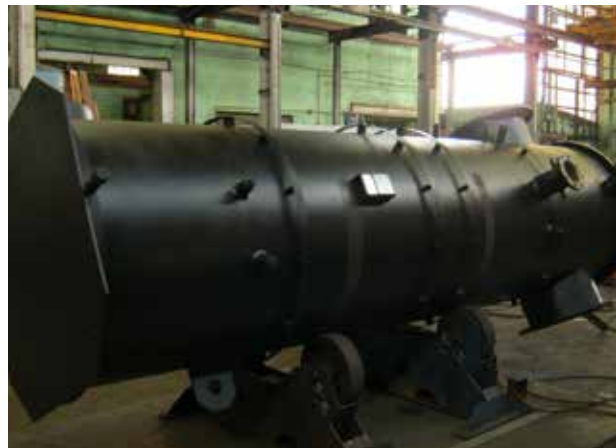
New Heat Recovery Unit in the factory.
