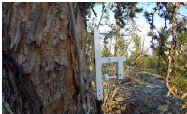
Dendrometer Installed on a jack pine.
