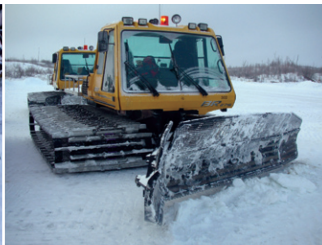
FIGURE 29. A low ground pressure vehicle, such as a snowcat, can be used for a first pass to compact snow on a winter road.
