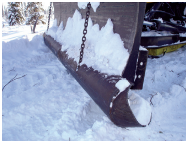
FIGURE 28. A smear blade raises the bulldozer blade off the ground surface.
