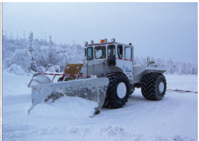
FIGURE 41. Clearing snow is part of routine winter road maintenance.
