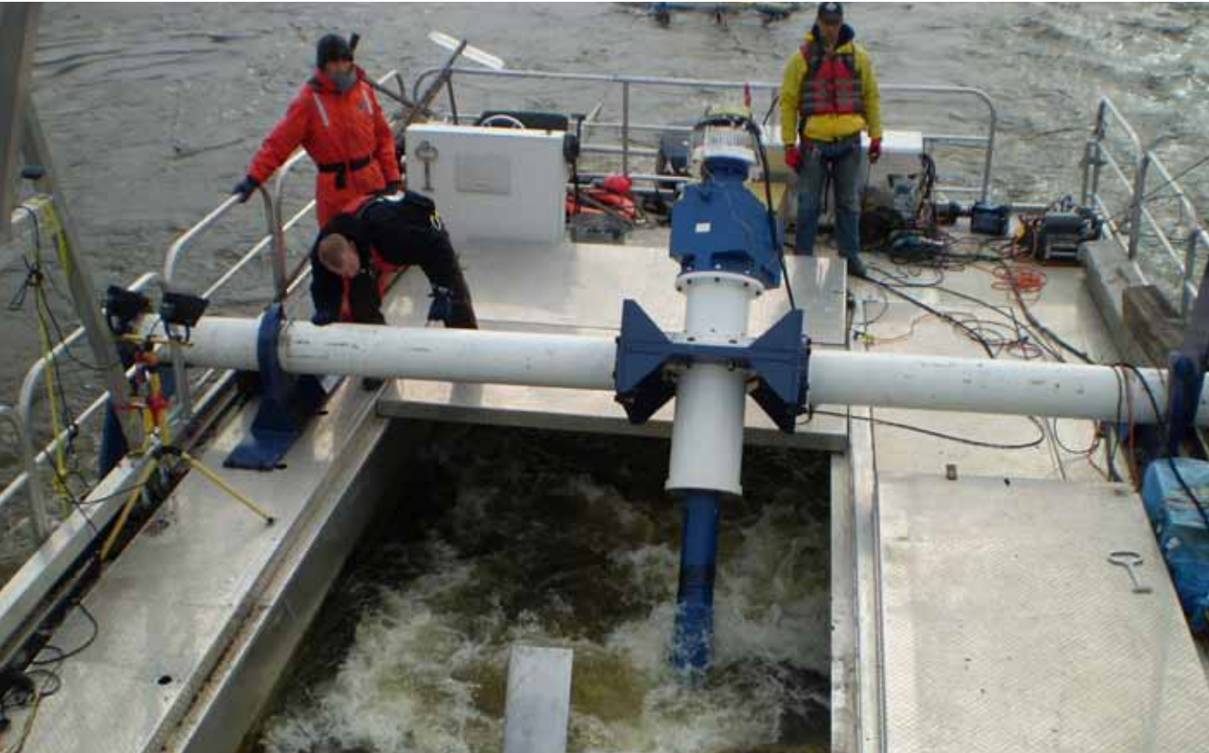
A 25 kilowatt hydrokinetic turbine at Pointe du Bois in Manitoba. A similar pilot project will be installed near Fort Simpson in the summer of 2010.
