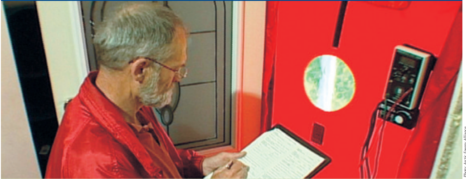
EnerGuide for Houses Audit: Doing a blower-door test to determine air infiltration.
