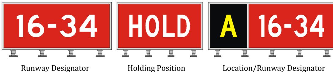
For airports within area of compass unreliability, the **runway designation sign** will include a letter “T” after the runway designator numbers, to indicate the “true north” heading of the runway rather than the “magnetic north” heading of the runway.
