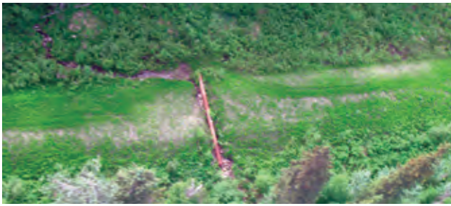
FIGURE 44. This reclaimed site is well contoured and revegetated, but the culvert should be removed.
