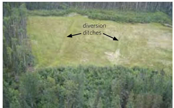
FIGURE 26. (top) A properly reclaimed campsite with all materials removed. Core sample boxes may remain in place.
