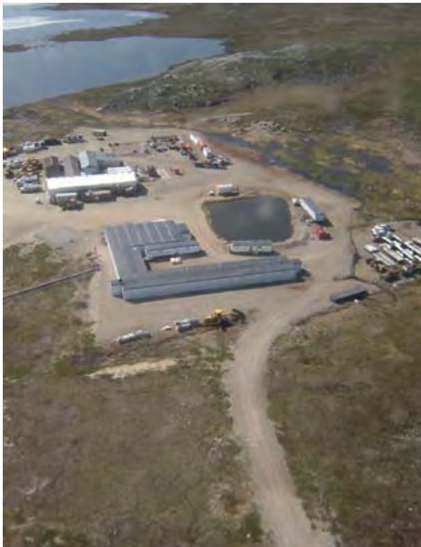
FIGURE 23. A large stationary camp with a sewage lagoon for waste-water treatment.
