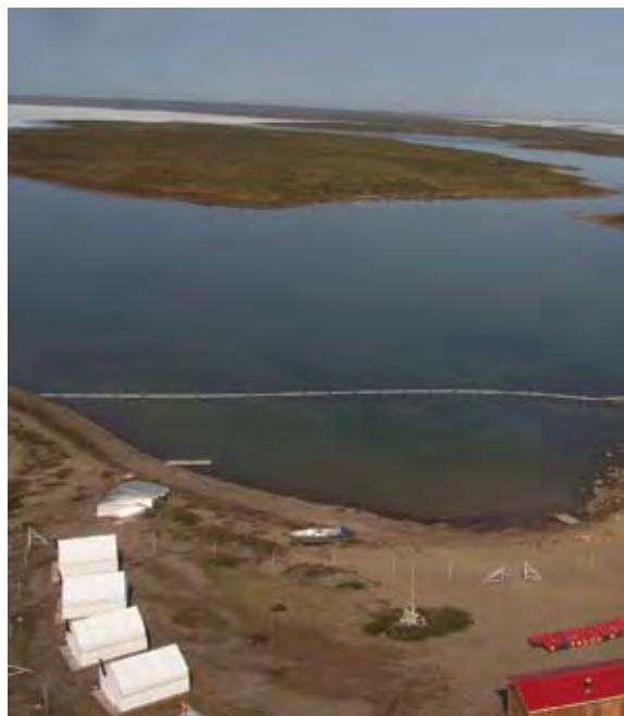
FIGURE 25. A spill-response kit should include absorbent booms to contain spills on water.
