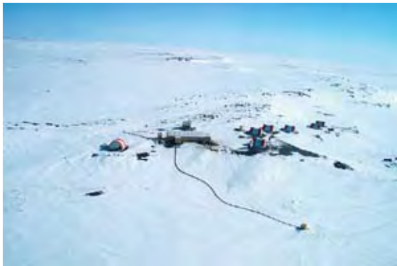
FIGURE 9. On the tundra, camps located on high ground require less snow removal.
