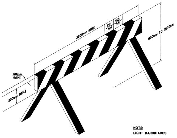
LIGHT BARRICADES MAY BE USED FOR WORKS OF SHORT DURATION TO PROVIDE THE CLOSURE OF A TRAFFIC LANE OR ROADWAY. THIS TYPE OF BARRICADE SHALL HAVE ALTERNATE ORANGE AND BLACK STRIPES AT 45°. ALL STRIPES SHALL BE 150mm IN WIDTH AND SHALL BE REFLECTORIZED OR ILLUMINATED TO INDICATE THE SAME COLOR AND SHAPE BY NIGHT AS BY DAY.
