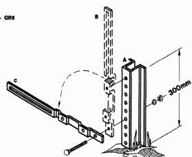
3. A - ATTACH SIGN POST WITH TWO 3/8" - 18 UNC x 2.0" BOLTS, NUTS, AND LOCKWASHERS IN BOTTOM AND FIFTH HOLES. (THESE CORRESPOND WITH SMALL SLOTS IN STRAP.
